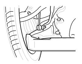
Note! Only the toe angle can be adjusted on the rear end but the camber angle must also be checked.
