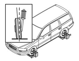
Lower the car on the turn table. Rock the car a few times. Check the values.
